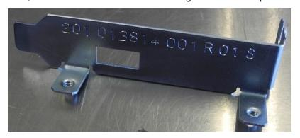
**4.** Align the SafeNet Luna PCIe HSM card with the vacant slot. You might need to introduce the tip of the card-hold-down bracket first (the silver-metal part along the back edge of the card), in order to properly align the card with the connector.
