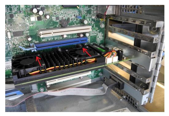
6. Secure the card hold-down bracket with a screw.
